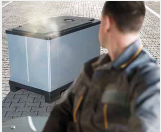
Minimising the rear view blind spot through short, low counterweight and a high seating position.
